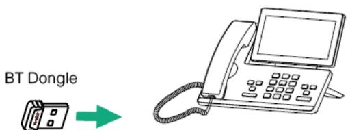
2. Press and hold the Bluetooth button for 2 seconds to enter the pairing mode.
